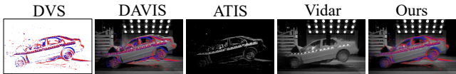
Figure 2: Visualization representation for the existing event cameras (i.e., DVS [15], DAVIS [2], ATIS [23], and Vidar [8]) and our visual sensing system. Note that, our work can effectively sense both dynamic events and visual textures using a unified representation.
